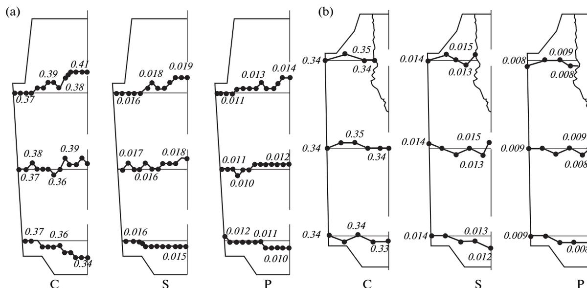
**Fig. 3.** Distributions of the carbon, sulfur, and phosphorus contents in various horizons of a reverse-taper ingot: (a) hot-tapped ingot 1.7 t in weight and (b) cold-tapped ingot 1.53 t in weight.
