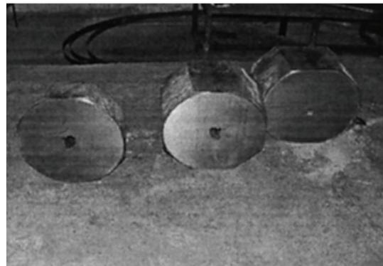
Fig. 2. Sections of a cold-tapped direct-taper ingot 2070 kg in weight.
