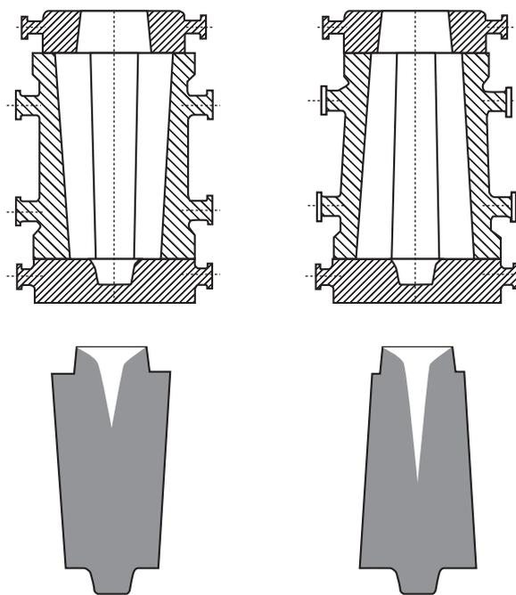
**Fig. 1.** Schematic diagram for the assembling of casting tool and the results of simulating shrinkage defects for cold-tapped ingots.
