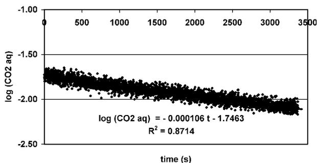
4 Kinetics of  $\text{CO}_2$  desorption from NaOH solution
