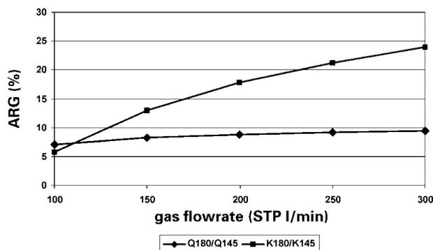
10 Circulation average relative gain (ARG) ( $Q_{180}/Q_{145}$ ) and degasification ARG ( $K_{180}/K_{145}$ ) as function of gas flowrate for two downleg diameters 180 and 145 mm
