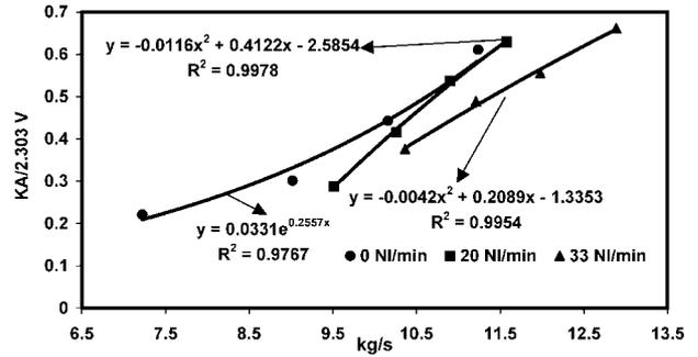
7 Lumped kinetic parameter versus circulation rate upon degassing for given rates of gas injection through porous plug as determined for water model
