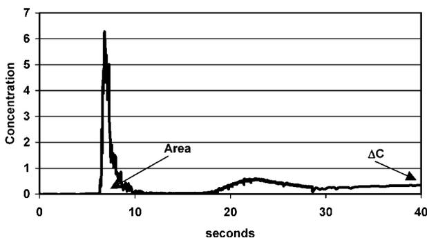
2 Typical concentration-time curve for calculation of circulation rate: (A: area under first peak,  $\Delta C$ : difference between final concentration and initial concentration of tracer)
