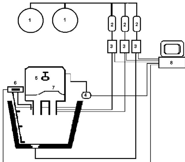
1: air compressor; 2: pressure regulator; 3: mass flow meter; 4: pressure transducer; 5: to vacuum pump; 6: conductivity meter; 7: injection point; 8: PC and A/D board
