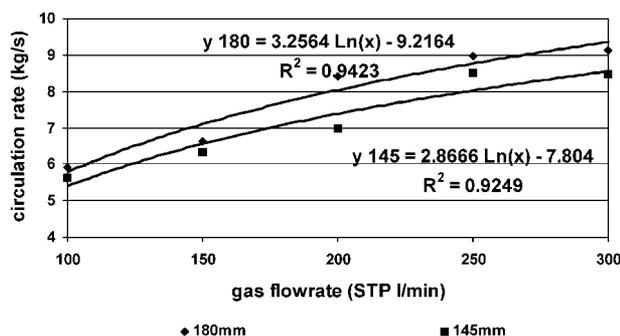
8 Liquid circulation rate versus gas flowrate for two downleg diameters 180 and 145 mm: upleg diameter is kept at 145 mm
