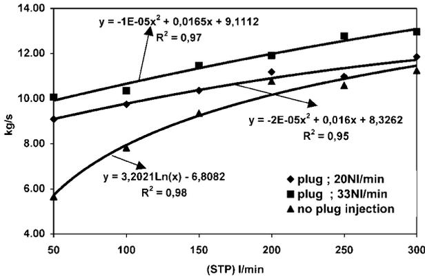
5 Effect of gas flowrate and bottom injection (porous plug) on circulation rate as determined for water model: x axis relates to gas injected through upleg only
