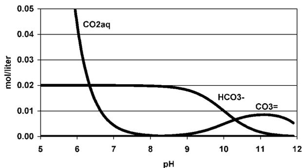
3 Equilibria between species in sodium hydroxide solution ( $[\text{NaOH}] = 0.02 \text{ M}$ ) and gas phase containing  $\text{CO}_2$
