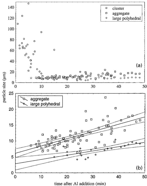
2 a Average sizes of clusters, aggregates, and large polyhedra versus time after aluminium addition in all three steel grades, and b increase in size of aggregates and large polyhedra in all heats: linear fits and 95% confidence bands are indicated
