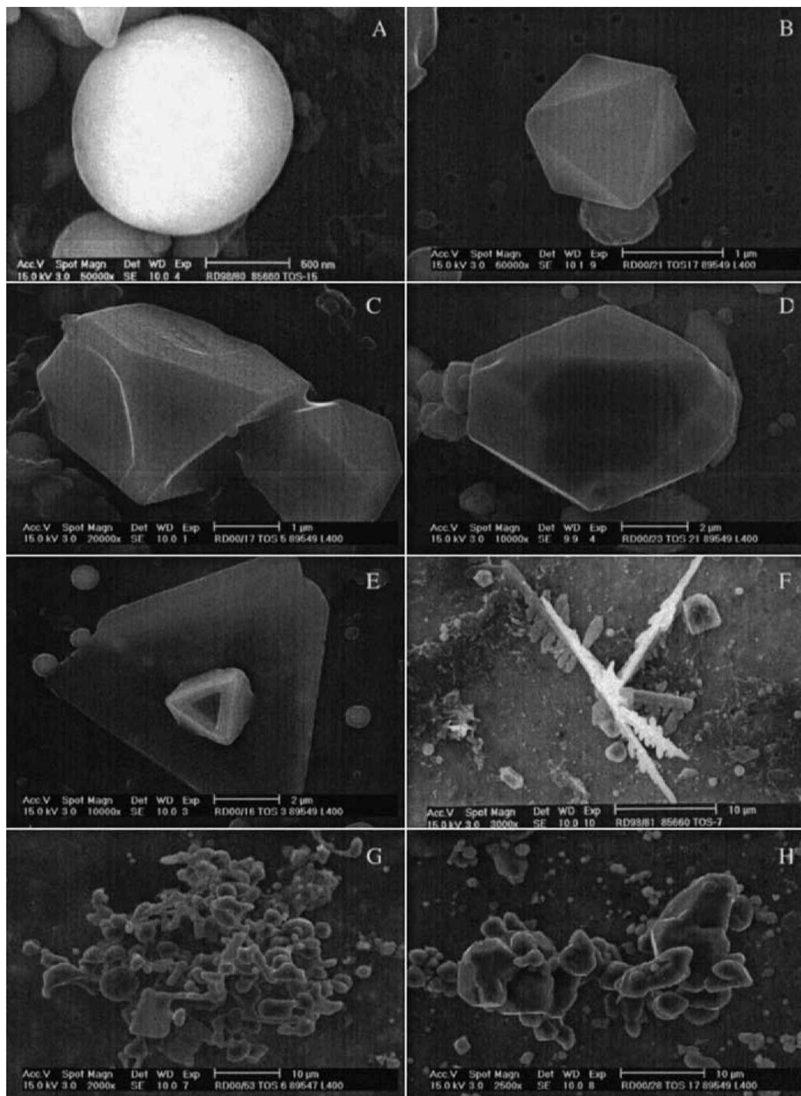
A small spherical inclusion; B octahedral inclusion; C small polyhedral inclusion; D large polyhedral inclusion; E platelike inclusion; F dendrite; G cluster; H aggregate
