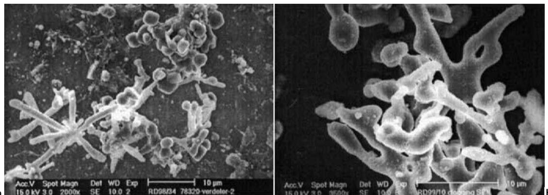
a cluster partially built up by dendrites in tundish; b clusters from clogging material
