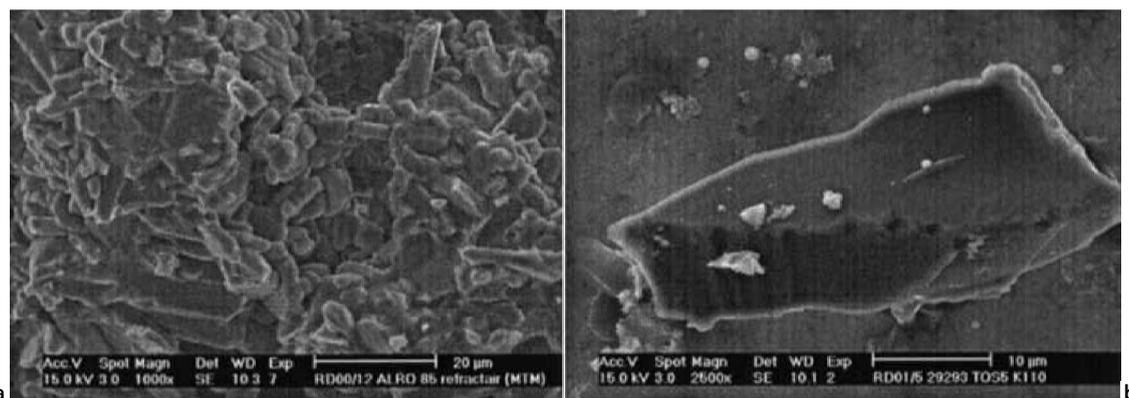
a surface of fresh fault in unused aluminium oxide refractory; b aluminium oxide particle found in steel sample
