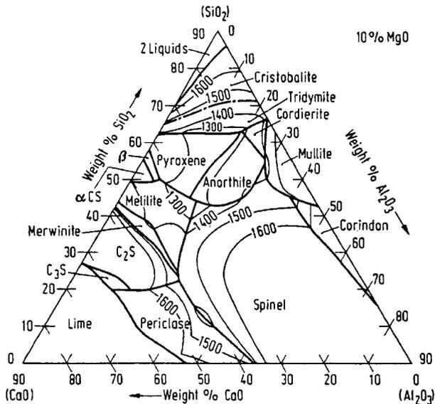
4 Phase diagram of Al<sub>2</sub>O<sub>3</sub>-CaO-MgO-SiO<sub>2</sub> system: after Ref. 11
