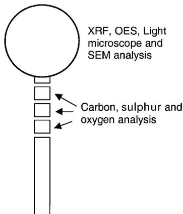
2 Steel sample in shape of lollipop: XRF X-ray fluorescence, OES optical emissions spectrometry
