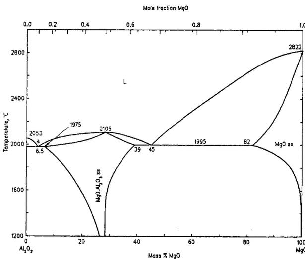
5 Phase diagram of Al<sub>2</sub>O<sub>3</sub>-MgO system: after Ref. 21
