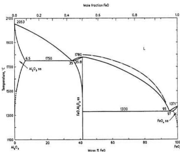
10 Phase diagram of Al<sub>2</sub>O<sub>3</sub>-FeO system: after Ref. 21
