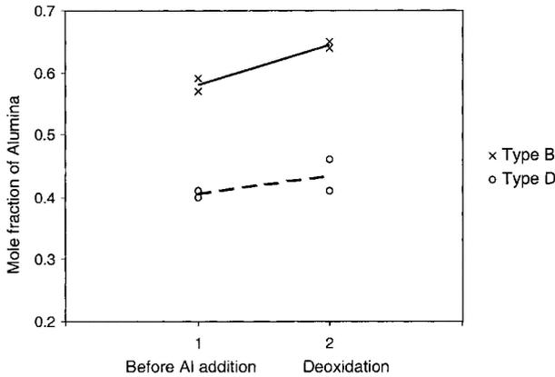
9 Variation of alumina content (mole fraction) in inclusions of type B and type D from start of ladle treatment to period of deoxidation
