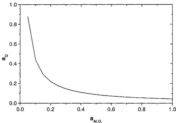
**8 Equilibrium oxygen activity a<sub>o</sub> as function of activity of alumina a<sub>Al<sub>2</sub>O<sub>3</sub></sub> at 1873 K for reaction (1): spinel Al<sub>2</sub>O<sub>3</sub>.FeO is stable in domain above curve**
