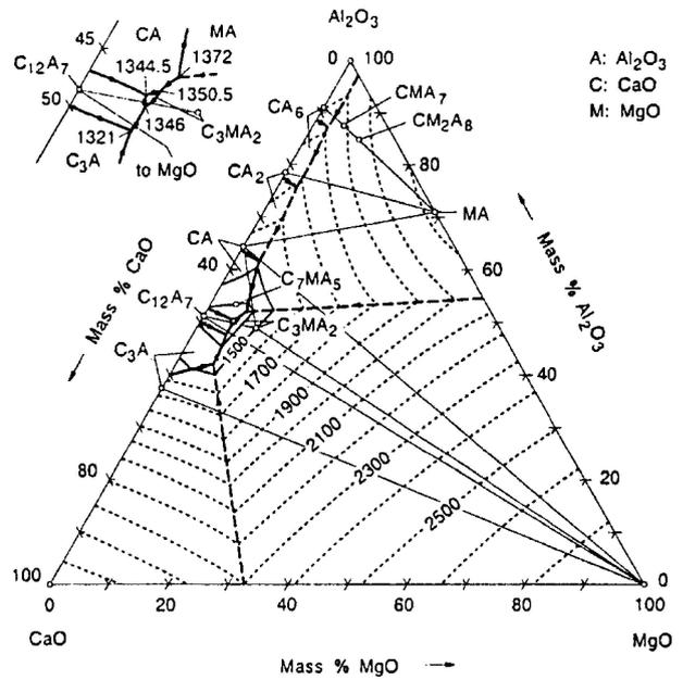
6 Phase diagram of Al<sub>2</sub>O<sub>3</sub>-CaO-MgO system: after Ref. 21
