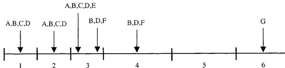
1: before deslagging; 2: after deslagging; 3: deoxidation; 4: alloying period; 5: degassing; 6: after degassing
