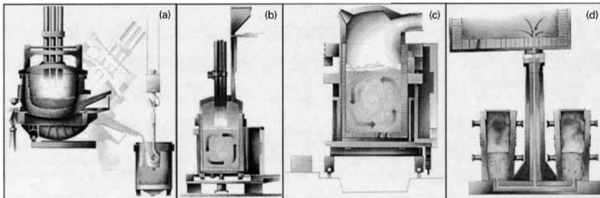
a electric arc furnace; b ladle furnace; c vacuum degassing; d uphill casting
